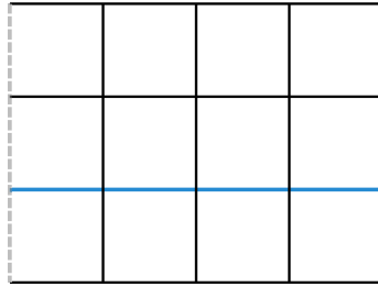
Figure 2.9: The surface code is defined on a L \times (L - 1) -square lattice. All edges (qubits) and vertices ( X -checks) in the lines defined by x = 0 and x = L are removed. A (relative) essential cycle corresponding to a logical Z -operator is highlighted in blue. The surface code is a [[L^2 + (L - 1)^2, 1, L]] -code.
